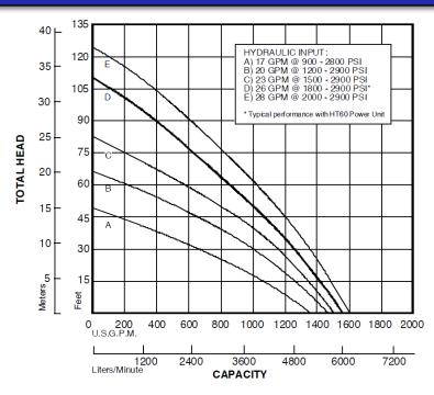
Curves are based on pumping water at 60°F. For performance curves other than shown above, consult factory.
