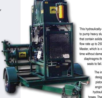
This hydraulically-driven, piston pumping system is designed to pump heavy sludges, slurries and other viscous materials that contain solids and impurities. The pumping system has a flow rate up to 250 gallons per minute. The self-priming Sludge Master, which is virtually leak proof, can dry run for a limited time without damage. It features low maintenance with no diaphragms that can burst under pressure or mechanical
